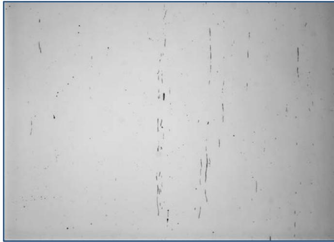
Micrograph showing MnS inclusions in steel
