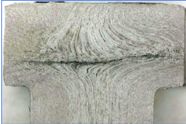
Macrograph of a forging burst
