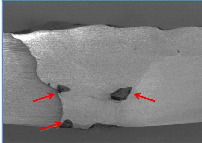
**Tungsten inclusions:** In the TIG process, the touching of the electrode to the weld metal may cause transfer of the tungsten particles into the weld metal. These inclusions are detected by x-ray and show up as bright particles since they are much denser than the steel. An example is shown below where the x-ray revealed the tungsten inclusions.
